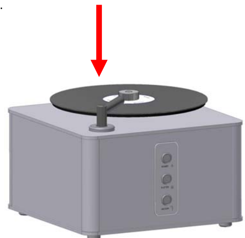
Pic. 4: Vacuum arm installation
